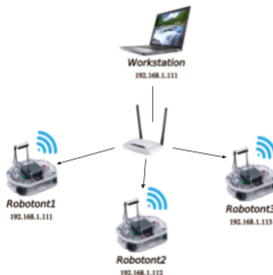
Figure 18: Network topology diagram of the configuration, each robot is automatically assigned a fixed IP address. They are all wirelessly connected to the same network and can be accessed via a single workstation.
