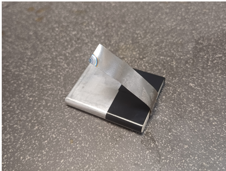
Figure 4.3. Li-ion cell after short test.
