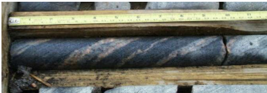
Figure 11. Measurement of leucosome widths in a drill core from the Estonian basement.
