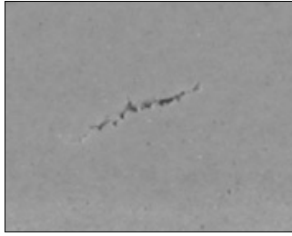
Figure 14. Formation of an initial subhorizontal crack. Actual size.
