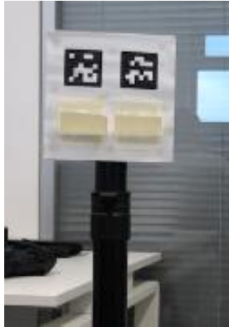
Figure 16. Calibration target with two tags.
