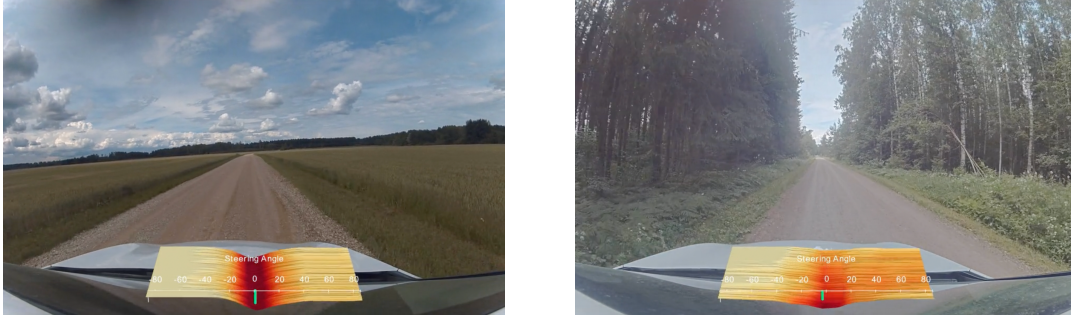
Figure 2. Visualization of the energy landscape across time on a recorded drive. The green pointer shows the predicted steering angle value at the current timestep. Left: the landscape has a clearly defined valley around 0 steering angle, representing high confidence. Right: the valley is about to disappear, replaced by a flatter region. Not shown here, the flat region, lasting for 7 seconds, was accompanied by the model drifting from the road, causing an intervention. The images were cropped arbitrarily and do not represent the model view.
