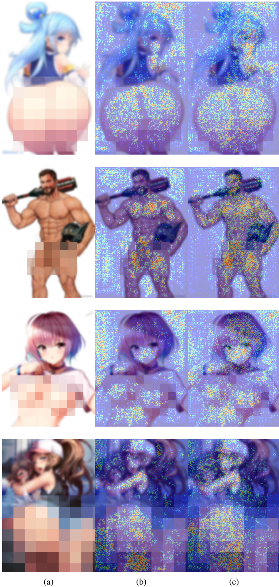
Figure 5.5: Network visualisation for Sexual Explicit Artwork . The first column depicts the original input image. The following columns are visualisation results respectively obtained using Guided Gradient-weighted Class Activation Map Saliency [4], Integrated Gradients Map [5].
