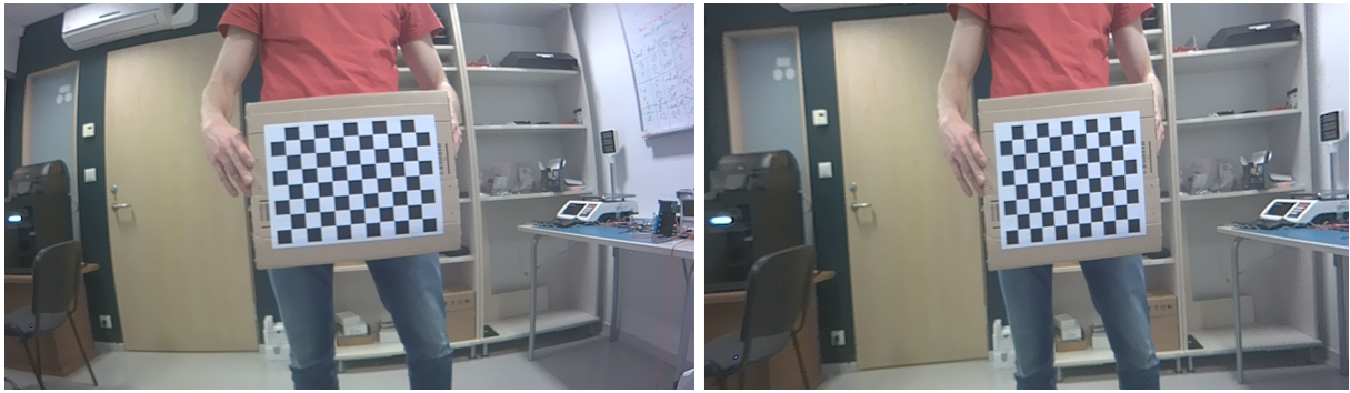
Figure 3.2: The left image shows the original distorted view as captured by the camera, while the right image displays the undistorted result after calibrating the camera.
