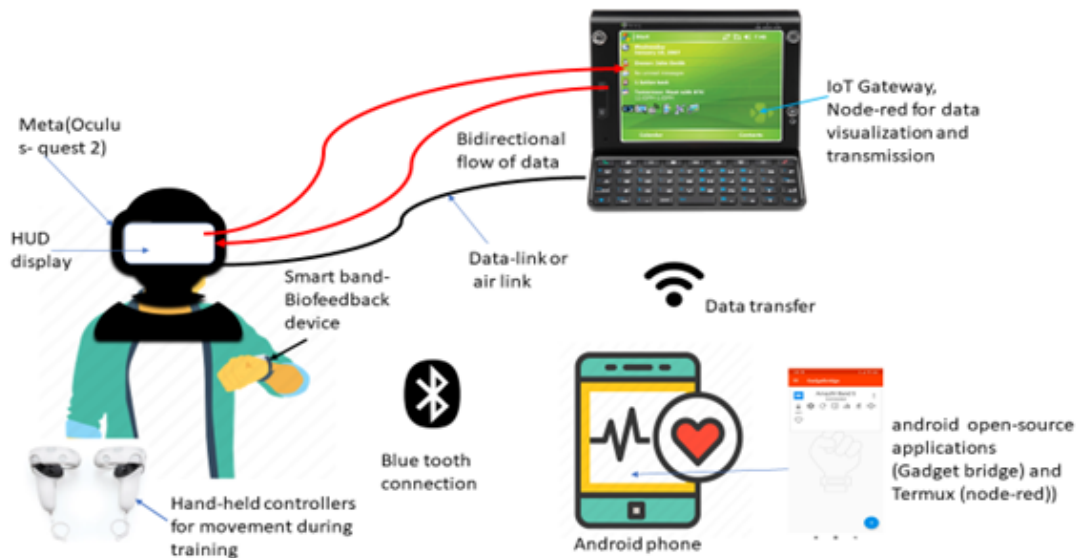
Figure 5. Architecture overview of biofeedback prototype
