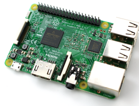
Figure 5. Raspberry Pi 3B. Gareth Halfacree from Bradford, UK, CC BY 2.0, via Wikimedia Commons.
