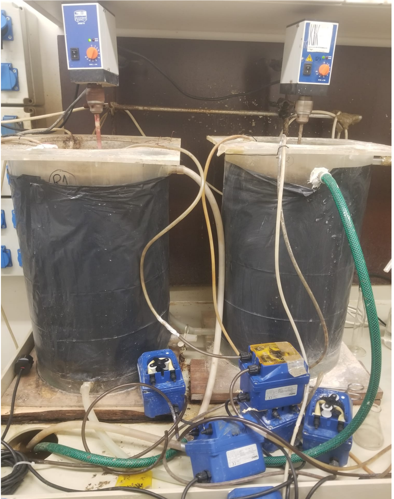
Figure 3. Schematic view showing two lab-scale MBBR reactor (20 L) set-up for anammox process at 22 0 C. Left side reactor was used for most of batch tests with pharmaceuticals.
