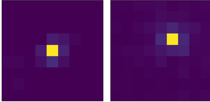
Figure 3: Signal amplitude samples for hits at (0, 0) and (20, 20) mm, respectively, with brighter color indicating higher amplitude increase.
