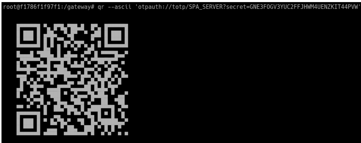
Figure 9. Encoding the TOTP secret in a QR code for transportation.
