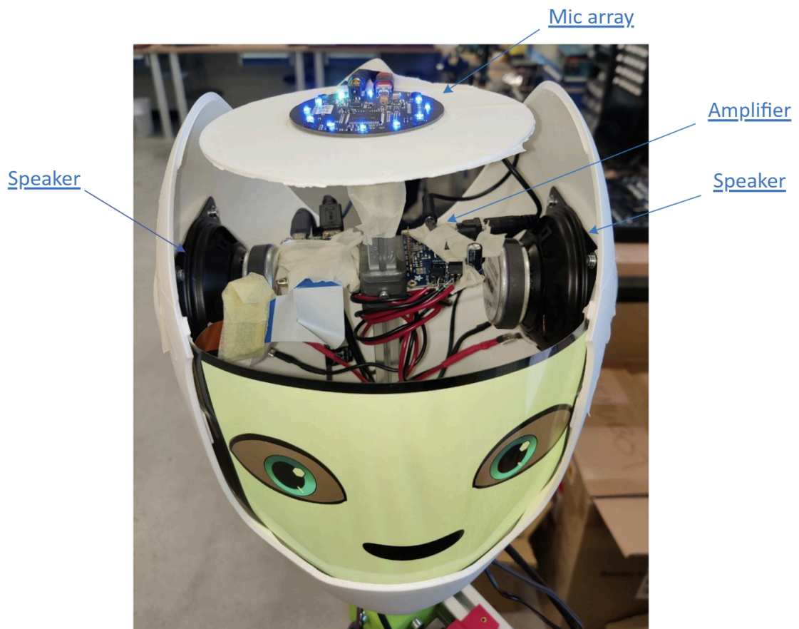
Fig. 18. The hardware assembly on the SemuBot robot
