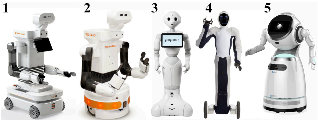
Figure 1: Humanoid robots with different wheelbases: 1 - Tiago with omnidirectional base; 2 - Tiago with differential drive base [7]; 3 - Pepper Humanoid [8]; 4 - EVE humanoid [9]; 5 - Cruzr robot [10]
