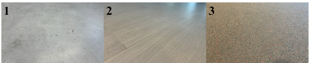
Figure 29: Tested drive surfaces: 1 - concrete floor; 2 - tile floor; 3 - carpet
