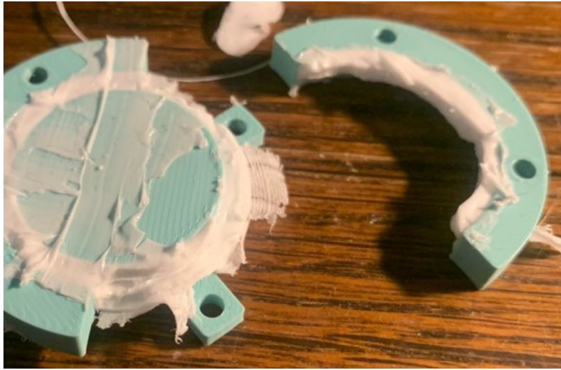
Figure 57: Removing dried caluk from a third iteration mould.
