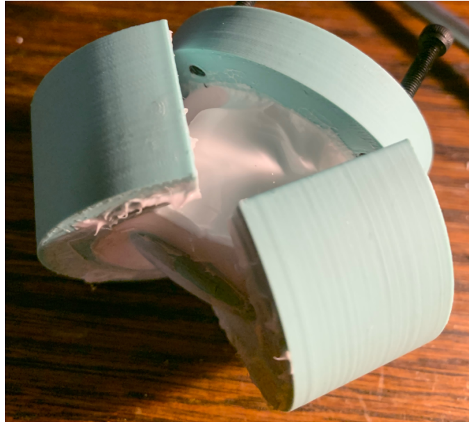
Figure 55: Unevenly dried caulk inside the second iteration of the mould.
