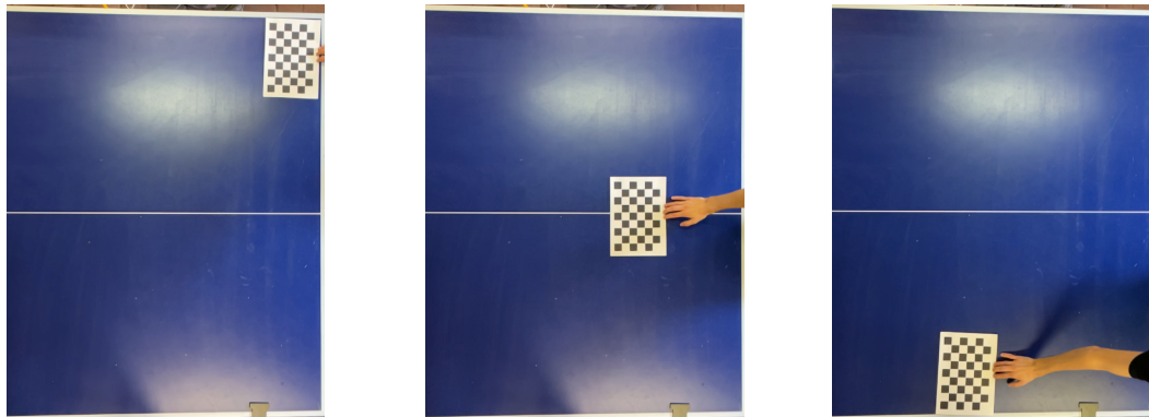
Figure 49: Gathering calibration data for resolving the camera's intrinsic and extrinsic properties for the automatic test setup. A 6x9 flat calibration chessboard is moved to various locations on the table, and recorded by a camera. Three sample locations are pictured.
