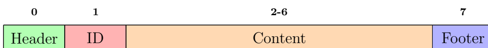
Figure 42: Structure of an individual 8-byte packet, consisting of a header (1 byte), an ID (1 byte), content (5 bytes), and a footer (1 byte).
