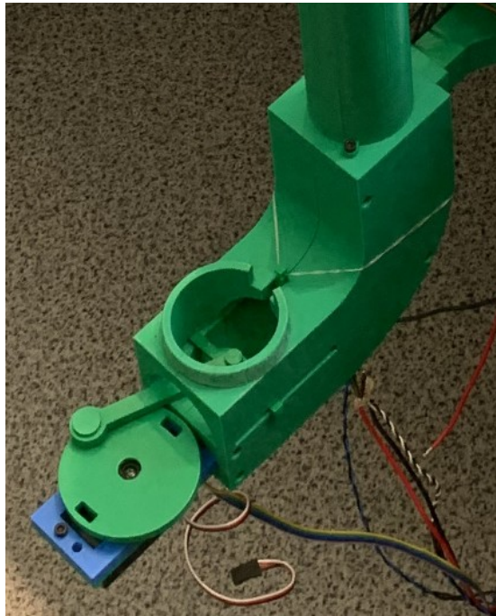
Figure 17: The second revision of the Ball Pusher. A clear rubber band is used to force the ball stopper into an upright position. A funnel (not depicted) can be pressure fit on top of the large opening to direct balls into the housing.
