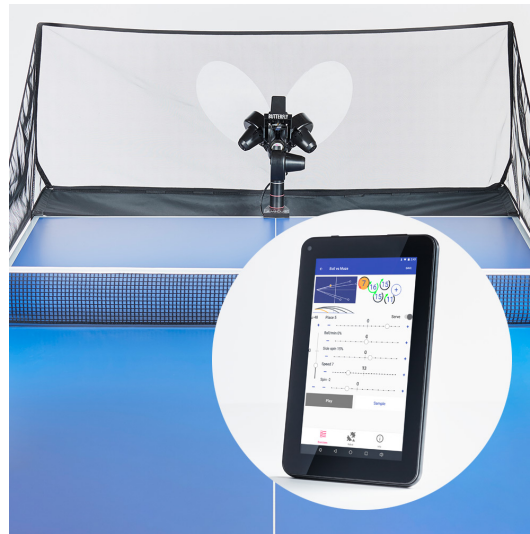
Figure 2: The AMICUS PRIME robot sold by Butterfly, mounted on a table tennis table. The robot can be controlled using the tablet shown in the foreground. A net behind the robot is used for reusing balls returned by the player. [9]
