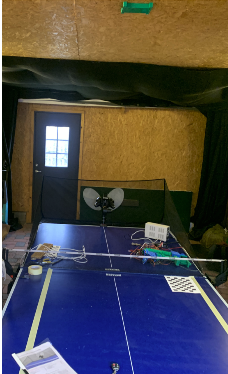
Figure 61: Butterfly AMICUS PRIME mounted on a table tennis table with the included ball catch net behind it. The launched balls were caught by hand and returned to the robot's side of the table. A roll of yellow masking tape holds down the piezoelectric element on the near side of the table for detecting ball bounces. A 3D printed smartphone camera (green) can be seen mounted to the wooden ceiling.
