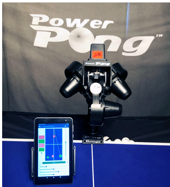
Figure 1: PowerPong's OMEGA robot mounted on a table tennis table with a ball collection net in the background. The robot can be controlled using the tablet shown in the foreground. [7]
