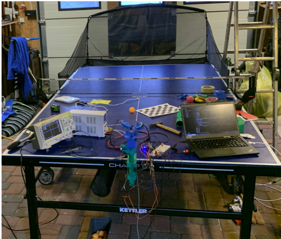
Figure 60: Rhea mounted on a table tennis table at a 10^\circ altitude angle. The launched balls are caught using a ball catch net ( JOOLA Carbon Graphite Ball Catch Net [54]) and returned under the table using a gutter for convenience. A roll of yellow masking tape holds down the piezoelectric element on the opposite side of the table for detecting ball bounces. A smartphone camera (not pictured) mounted on the ceiling records the landing locations of the balls.
