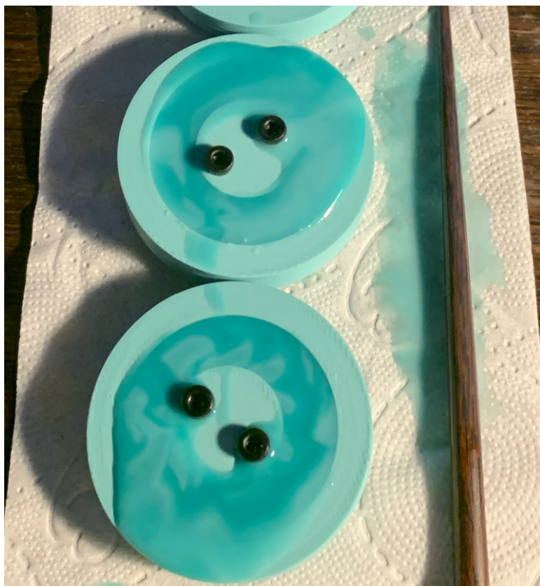
Figure 59: Fifth iteration the moulds, poured with Shore A 22 polysiloxane.
