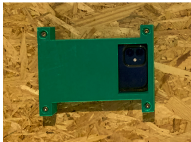
Figure 48: 3D printed smartphone mount located above the table tennis table, fixed to a wooden ceiling using screws. The smartphone's camera provides a top-down view of one side of the table and it can be slid in and out of the mount.
