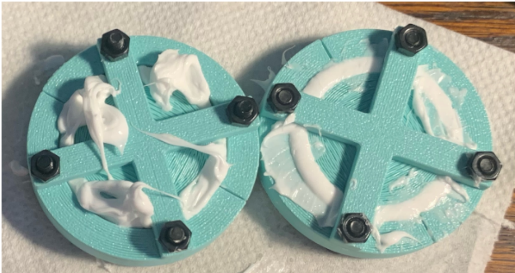
Figure 56: Caulk drying inside third iteration moulds, inner surfaces lubricated with oil.
