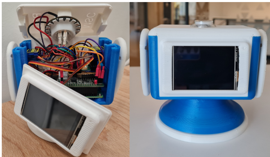
Figure 4.13: Internal and external looks of the final 3D-printed RSC prototype.
