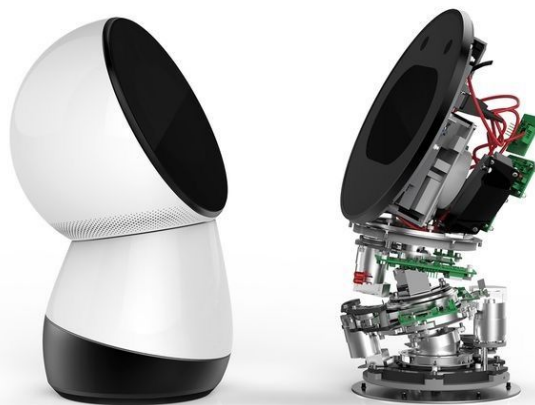
Figure 2.2: Jibo's external and internals [27]
