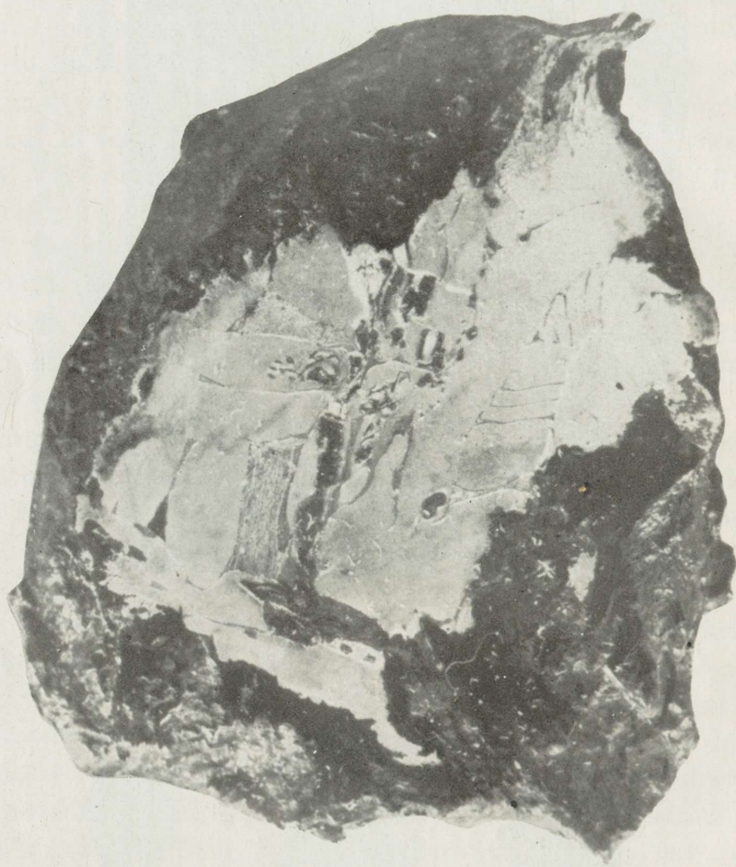
Fig. 16. Polished and etched surface, showing signs of crystalline structure in the biggest sample found in crater Nr. 2 \times 3. Photograph by author.
