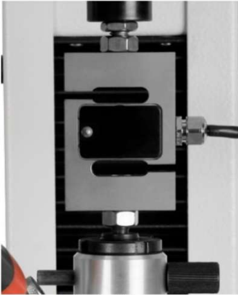
Fig. 6: load cell/ force sensor
