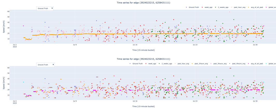
Figure 10. Data imputation methods. The top image shows a data imputation method that resulted in a fallback to a constant value. The bottom image, corresponding to the final solution used, breaks the pattern of a straight line.
