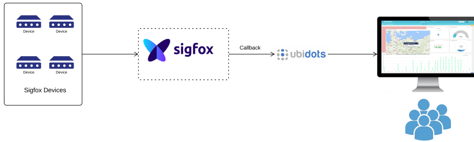
(a) Sigfox and Ubidots basic architecture
