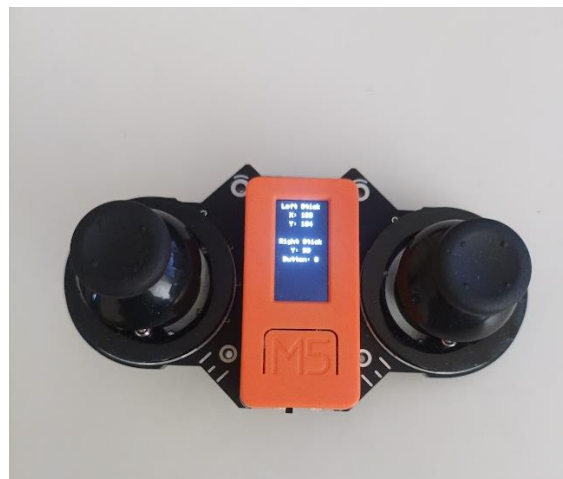
Figure 2. M5StickC and JoyC Omnidirectional Controller.
