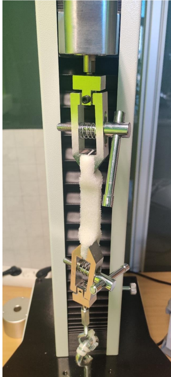
Figure 11. Dumbbell specimen in the grips of the Motorized Test Stand model AEL-A-1000.
