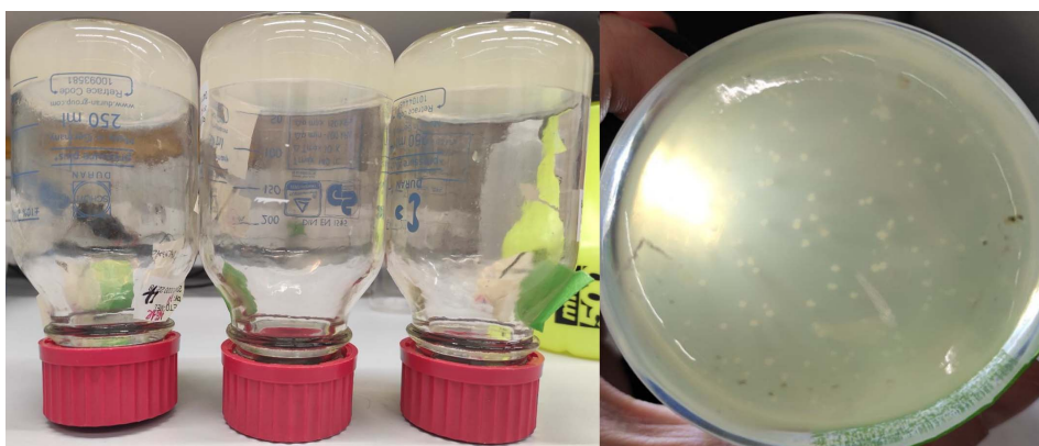
Figure 11. Agar system developed in GasFermTEC for isolation of ALE isolates in autotrophic growth conditions.
