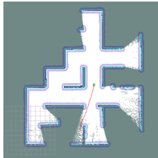
Figure 30. Collaborative Mapping Trial: Map Generated by Robot2 Prior to the first rendezvous
