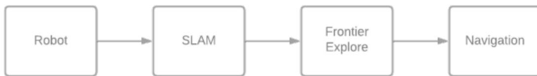
Figure 13. Block Diagram Representation Of Robot Exploration
