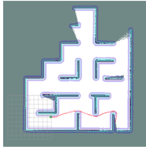
Figure 27. Independent Mapping Trial: Map Generated by Robot2 after a time T of exploration
