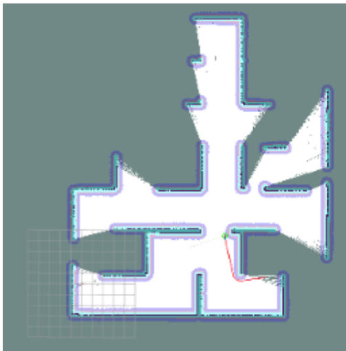
Figure 29. Collaborative Mapping Trial: Map Generated by Robot1 Prior to the first rendezvous
