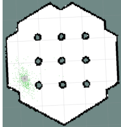
Figure 10. AMCL Algorithm after navigating for few seconds
