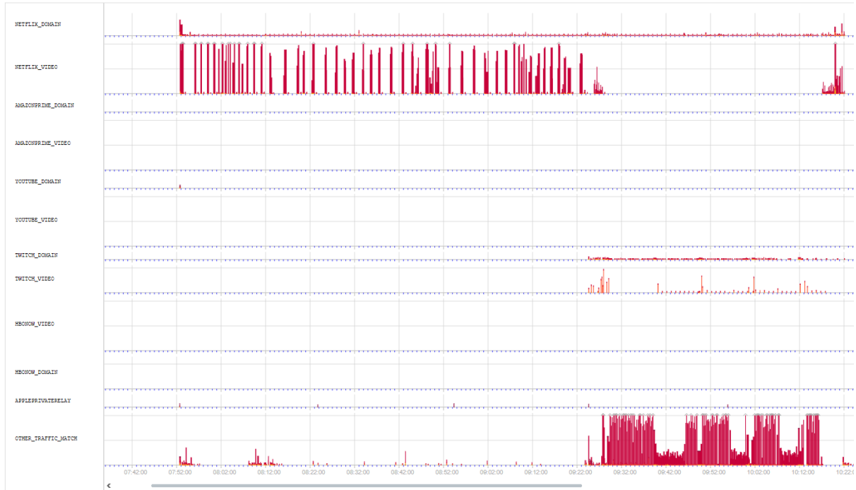
Figure 1.3: Example of a background app(Netflix) still generating data on the network while a parallel one is playing (Twitch). Also note the iOS Netflix bufferization pattern, different from the first example.
