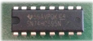
Joonis 40. 74HC595 8-bitine nihkeregister
