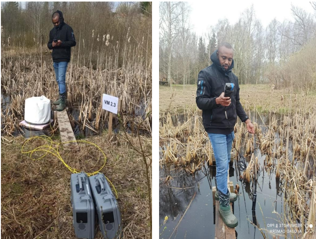
Figure 4: Author in the field, measuring CH 4 gas and water parameters using the LI-7810 trace gas analyzer (left) and YSI ProDSS (right).
