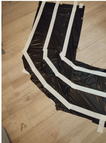
Figure 6.1: Picture of an extremity of the open circuit, displaying the setup of a black plastic bag over a clear floor and white tape to structure the track.
