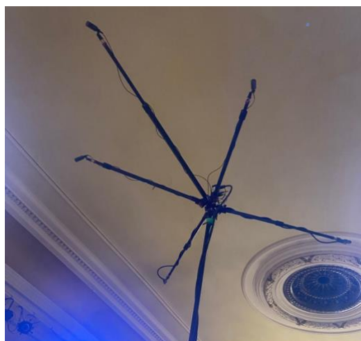
Figure 4. Decca tree array used in the trio recording
