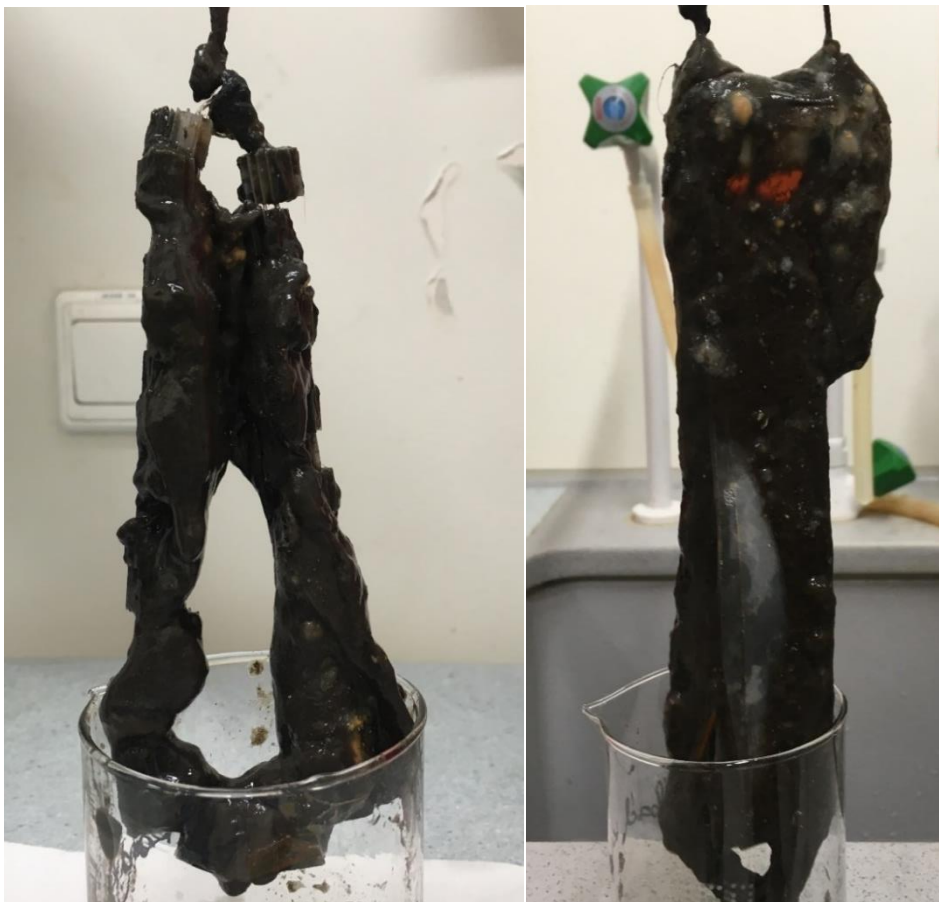
Photo 4. Bioflow 9 biofilm carriers (left) and on the right PE strips (right) after the second phase
