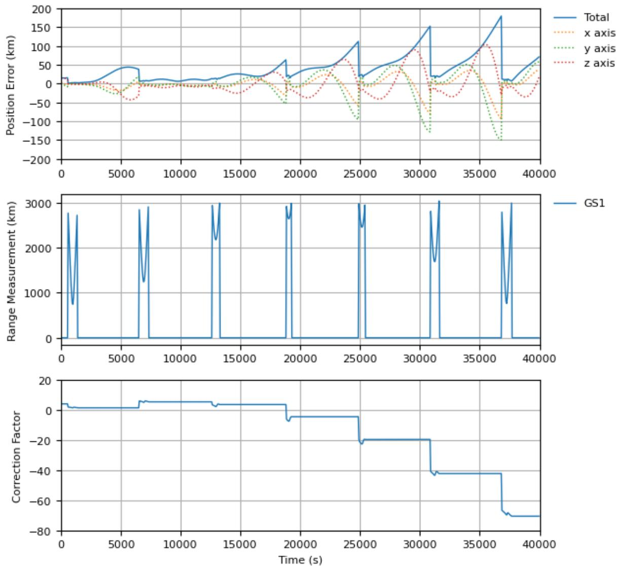
Figure 4.9: Position error, single ground station ranging
