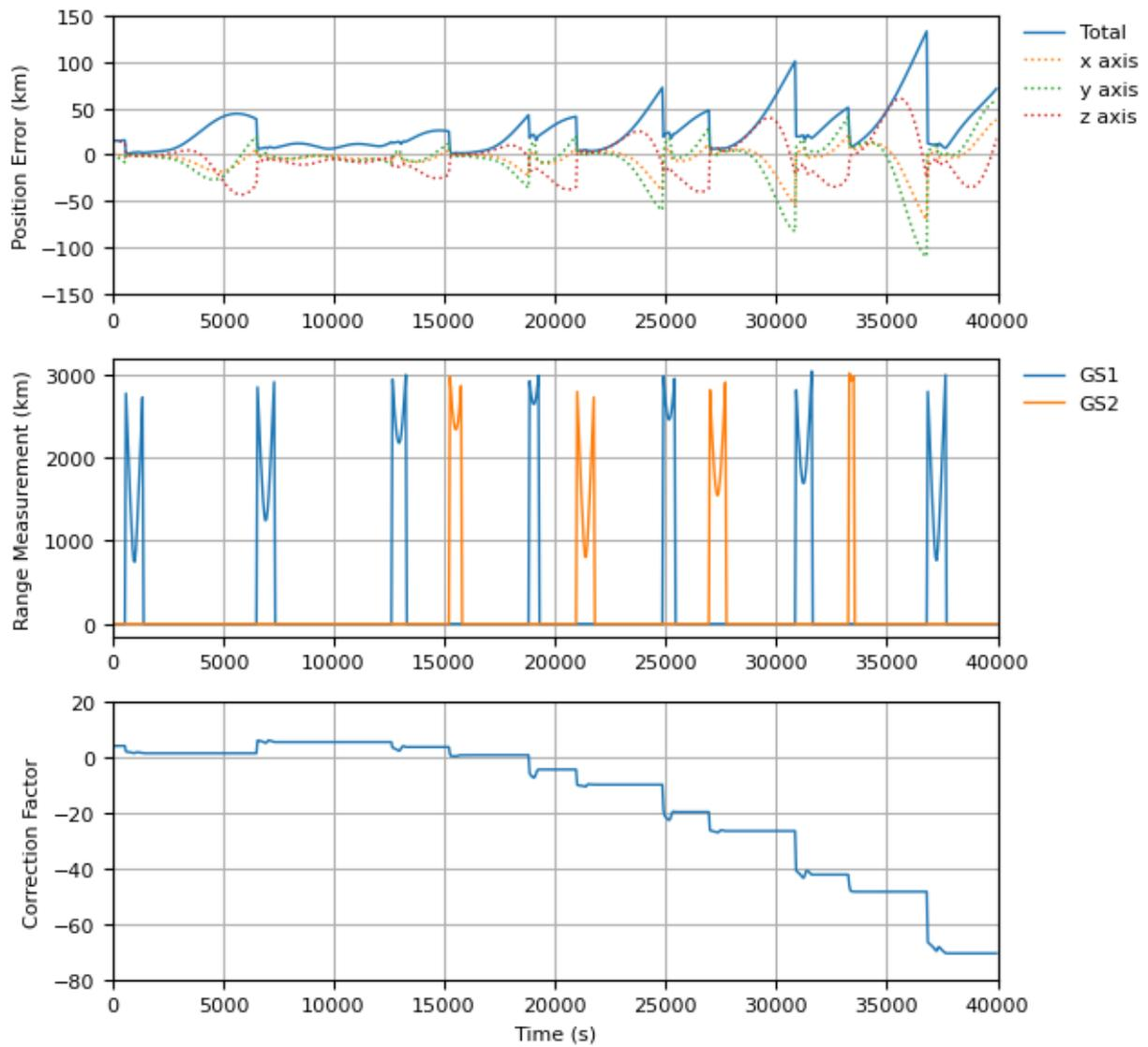
Figure 4.10: Position error, two ground stations ranging
