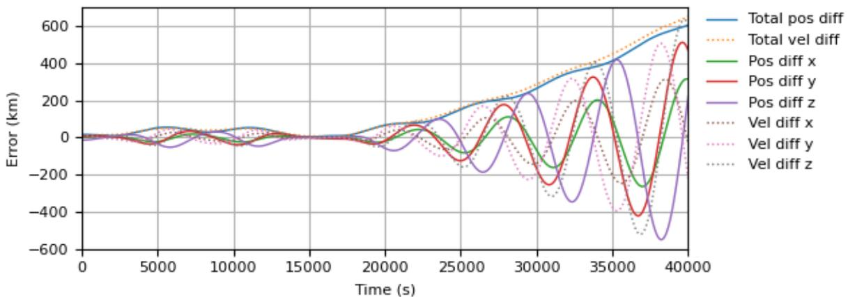
Figure 4.8: Orbital motion error, no ranging
