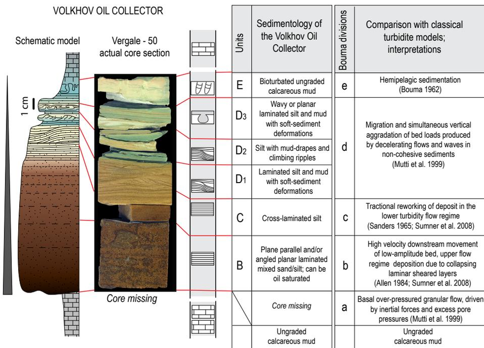
**Figure 5.** Schematic cross-section and photograph of the Volkhov Oil Collector in the Vergale-50 core section. The sedimentary textures are compared with the classical turbidite model by Bouma (1962). The elongated arrow in front of the schematic model indicates smooth grain-size decrease from the bottom to the top of the bed. (Modified from Põldsaar et al. 2019 – PAPER III).
