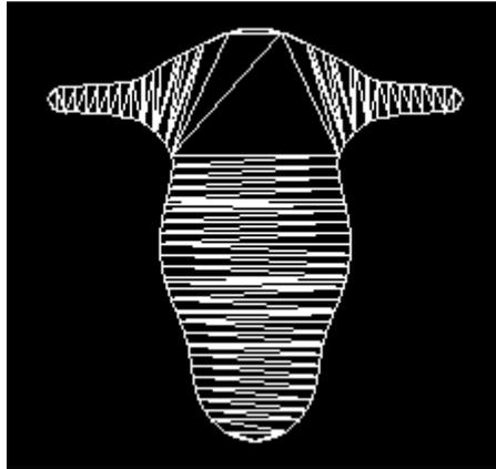
Figure 20. Example of triangulation using only the outline.
