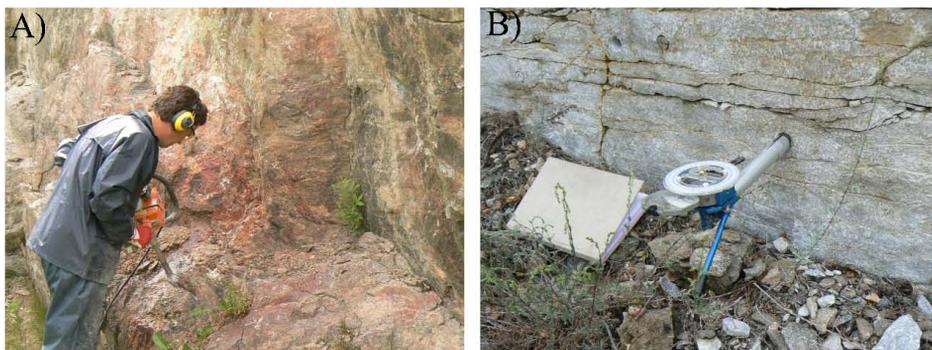
**Fig. 2.** (A) Sampling at Rajamäki with the gasoline drill. (B) Core orienting with sun and magnetic compass at Kallasto.
