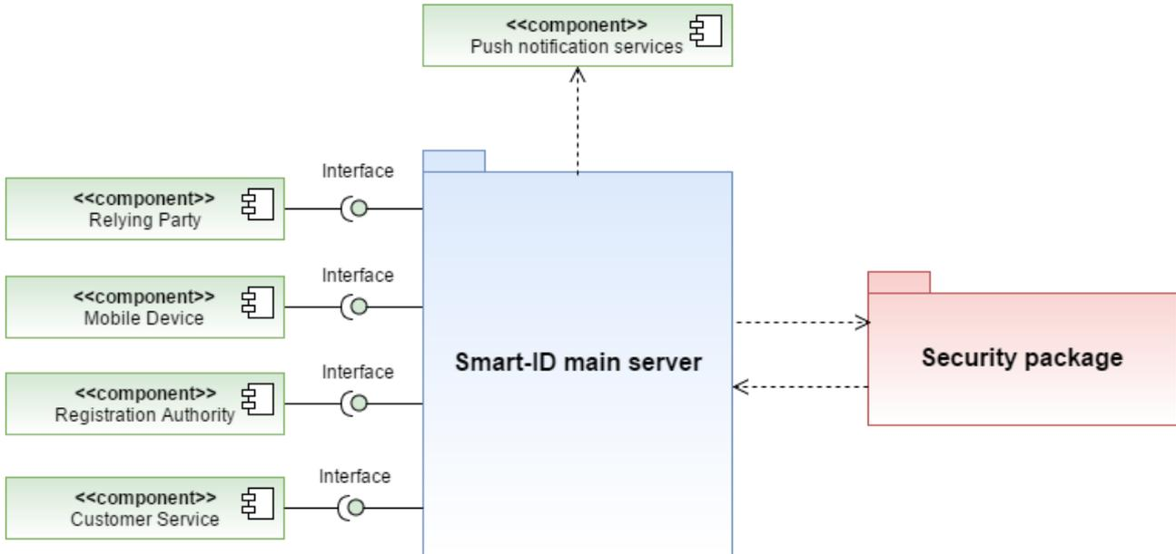
Figure 1 - Simplified Smart-ID internal architecture and relationships
