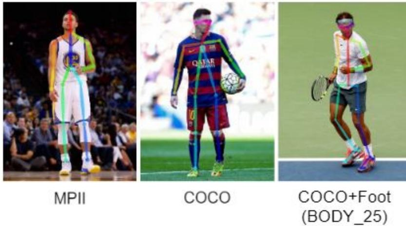
**Figure 9.** Three different body models, originating from different datasets [28]. MPII - Max Planck Institute for Informatics dataset. COCO - Common Objects in COntext [29] dataset.
