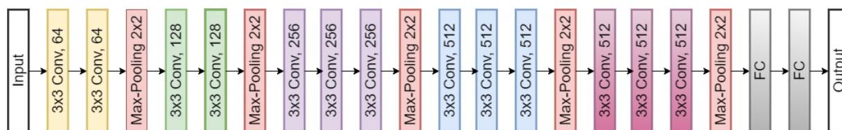
Figure 6. The structure of the VGG-16 model.
