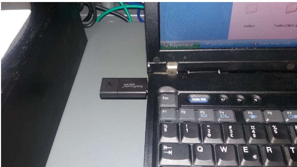
Picture 3. The cloned Tosibox key has been plugged to the laptop.
