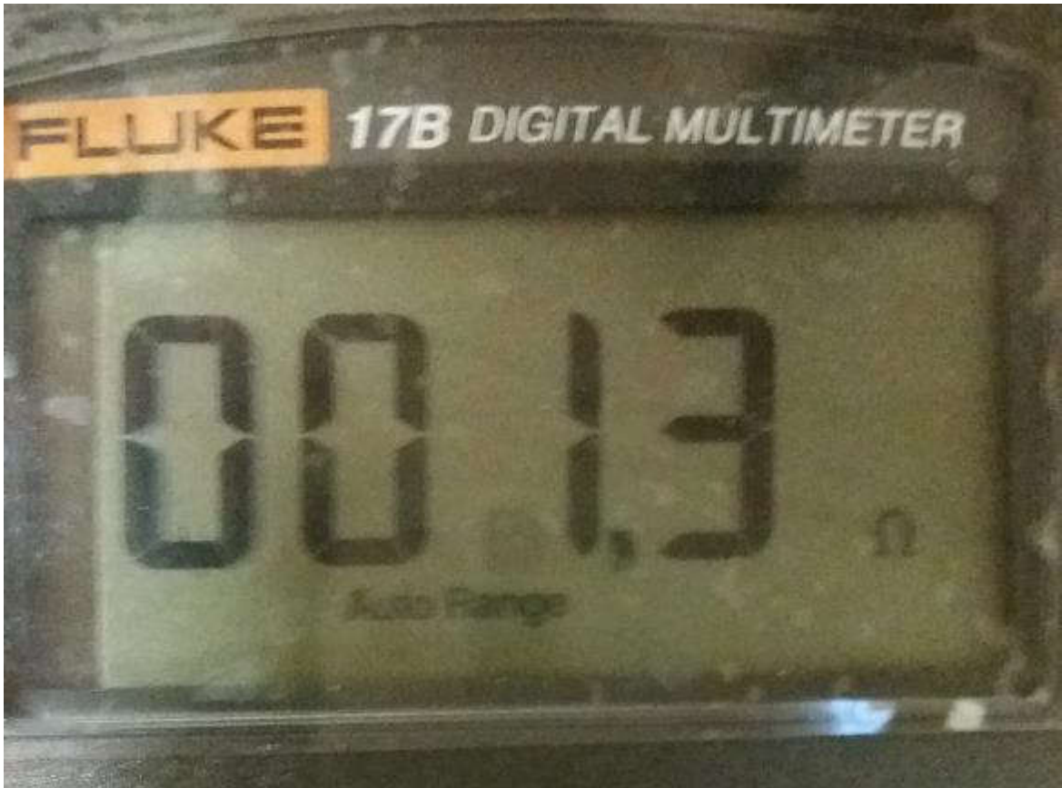
Picture 4. The resistor value which causes the actuator to go full open position.
