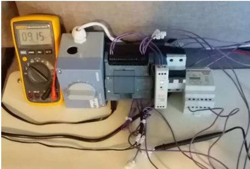
Figure 2. The Siemens S7 experimental environment. Photographer: Mikko Luomala.
