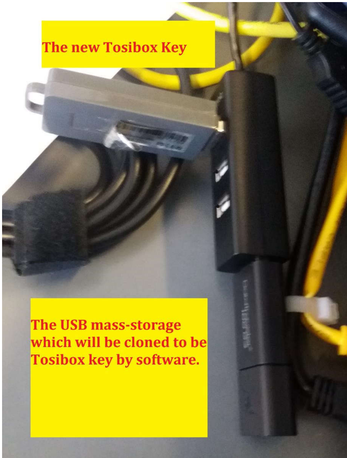
Picture 7. The new Tosibox key and USB drive which will be cloned.
