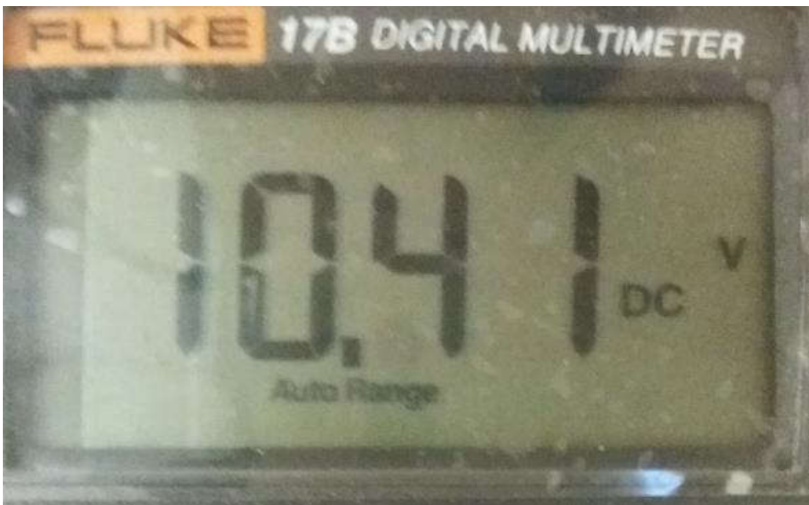
Picture 5. The voltage value when the SQS65 Siemens has been set as full open (Position 10).
