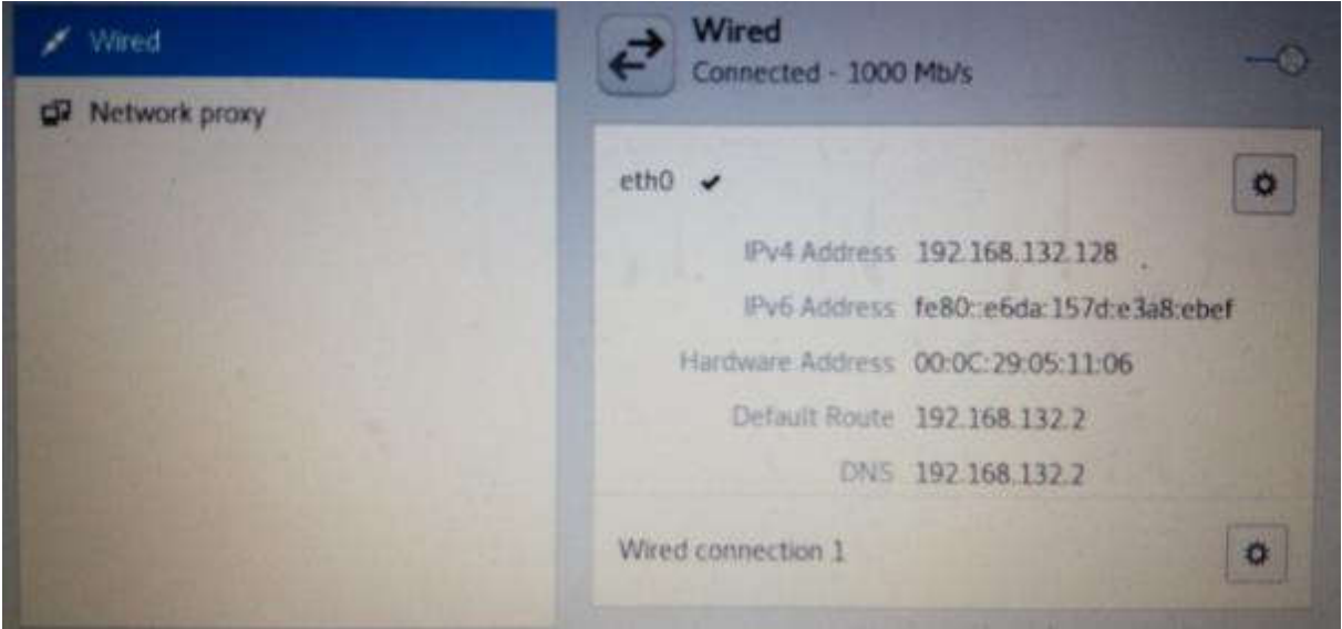
Figure 6. The Kali Linux obtain automatically IPv4 address from VMware Player 12 DHCP server. Photographer: Mikko Luomala.
